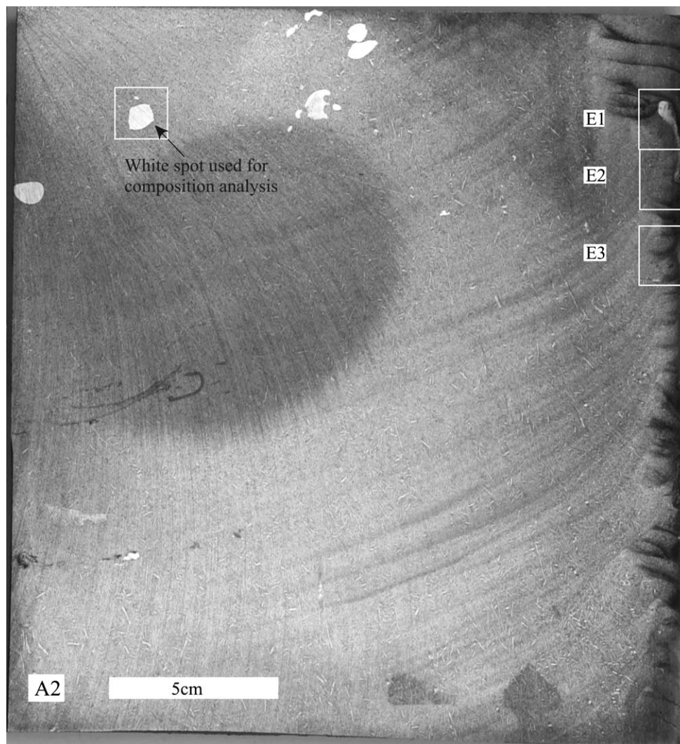
Figure 2 Slice A2, showing white spots. A close up of the region containing sample locations E1, E2 and E3 is shown in Fig. 5.
